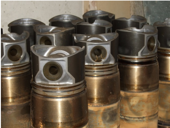
Figure 28: Vital for reliable operation is the regular overhaul of the CHP unit. In the picture: Engine cylinder pistons. Photo: F. Gerlach, MEP.
