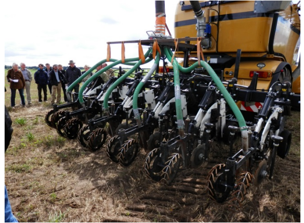
Figure 16: Slurry injection technology reduces ammonia emissions, thus improving nutrient recycling and reducing air pollution. Photo: N. Hölzer, MEP.
