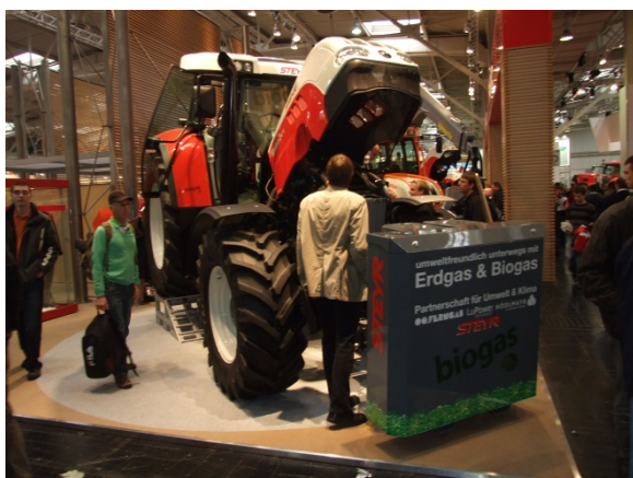
Figure 30: The first Biogas-powered tractors attract attention at trade fairs and on the fields. Upgraded biogas is stored in tanks under floor and optionally at the front. Photo: F. Gerlach, MEP.
